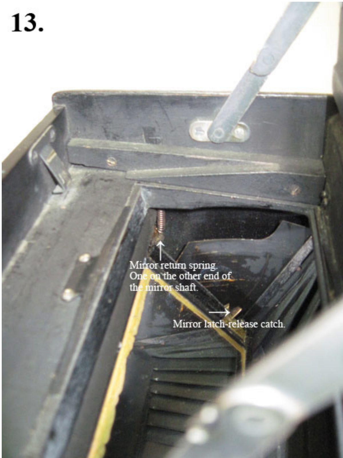
Mirror return spring and latch detail.
